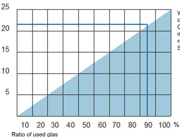
With an average ratio of 84,85 % Used Glass in 2014, melting-energy was reduced by 21,2 % in St.Prex.
